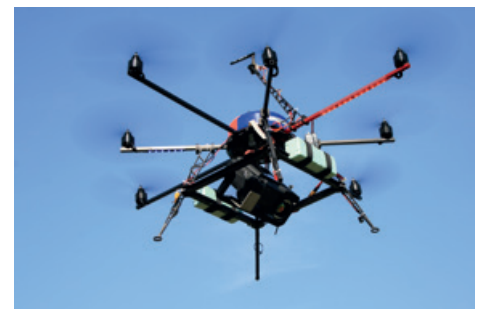
The drone consists of an octocopter, the FLIR T620 and a vertically tilting camera fastener with a total weight well under 5 kg.
