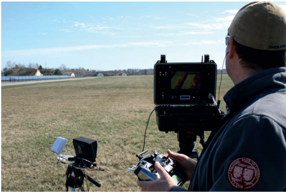
Mario Hambsch with the drone's remote control and the measuring kit, on the monitor on which the live stream is displayed. The infrared live stream is transmitted to the ground station on an ongoing basis, recorded by a digital recorder and displayed on the monitor of a special measuring kit. On the left side of the tripod: the antenna for the connection to the drone and the thermal imaging camera.
